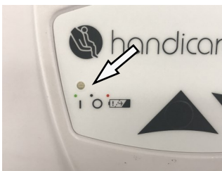
Figure 4B - The indicator light of the lift is normally off when not in use.
