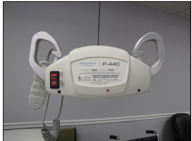
Figure 17B - P-440 (303073) with extended hooks (637045) turned upwards.
