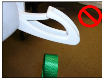
Figure 5 - Sling loop separated from the P-440 carry bar hook.
