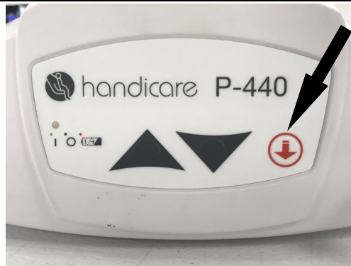
Figure 14B –RED emergency lowering button located on middle of the front of the lift.
