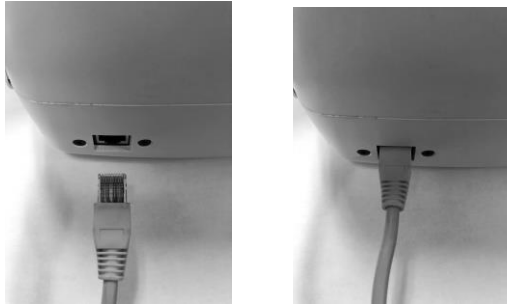
Figure 3: Hand Control connector with latch being inserted into lift connector
