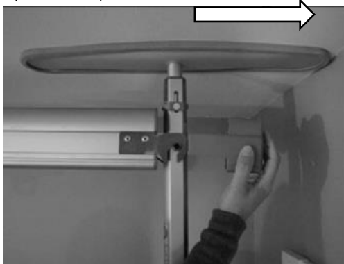
Figure 32: Remove the End Caps from Both Posts
