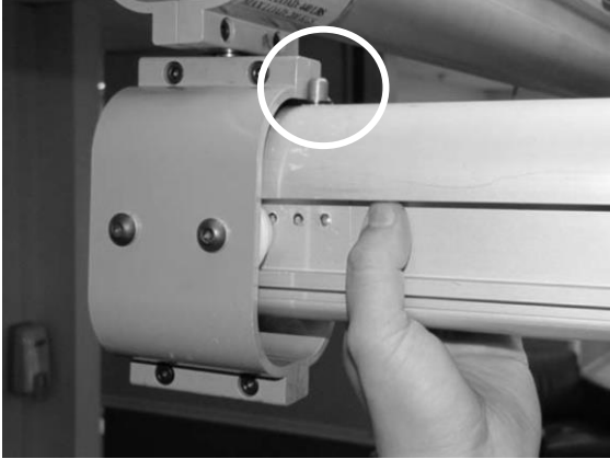
Figure 27: Traverse Track in the Trolley (Pin Against the Trolley)
