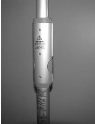
Figure 43: Level and Safety Lock at Original Positions
