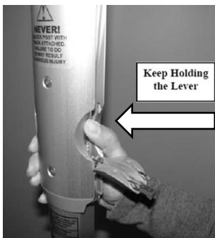
Figure 36: Release Pressure from the Ratchet
