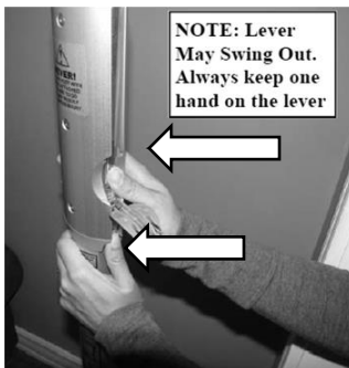
Figure 37: Push and Hold the Ratchet
