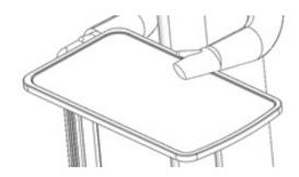
Gently lower the table by placing one hand on the table top while using the other for controlling the release handle.
