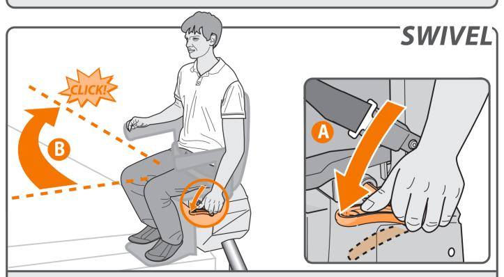
The lift stops automatically at the end of the rail. You can now swivel the seat manually, making it easier to get on and off. To do this, push down the lever{A}. Swivel the seat until you hear a 'click'. The seat is now in the correct position{B}.
