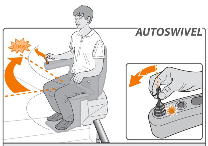
The AUTOMATIC SWIVEL SEAT option lets you swivel the seat automatically to face the direction you are going to walk in. To do this, push and hold the joystick in the upwards direction.
