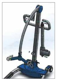
5. Attach the actuator to the lifter with cotter pins as shown above.
