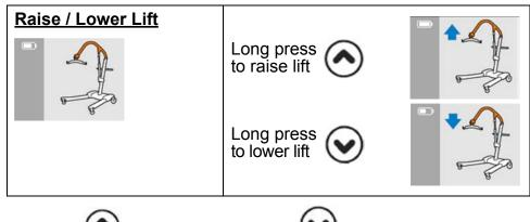
1. Press the  $\bigcirc$  button to raise or the  $\bigcirc$  button to lower the lift.
