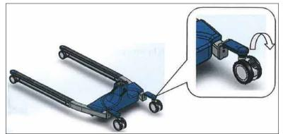
1. Engage the lift brakes as shown above.
