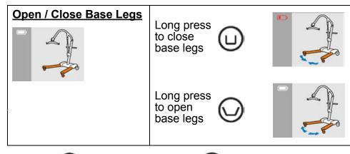
2. Press the  $\bigcirc$  button to open or the  $\bigcirc$  button to close the lift base legs.
