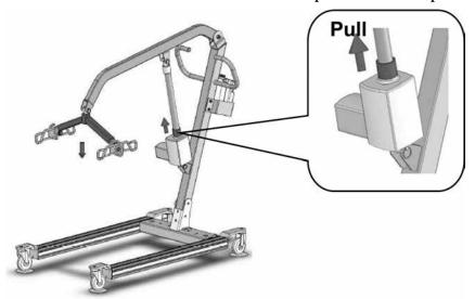
The quick release is available with a manual activation where a finger grip is mounted on the actuator. When pulling the finger grip the declutching is activated. Pull up the red emergency tab approximately one half inch using normal force. The actuator will then lower itself safely down. The lowering device will not lower unless weight is being applied.
