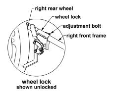
▲ WARNING: Ensure wheel locks are adjusted so they lock in place appropriately before occupying or operating wheelchair.
