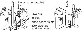
Step 4: Assemble lower holder bracket to lower rail
