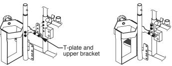
Step 3: Install T-plate on inside of frame
