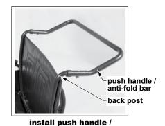
2. Install the nuts and bolts that secure the push handle / antifold bar on both sides as shown at right. Use an M10 wrench and M4 hex key to tighten.
