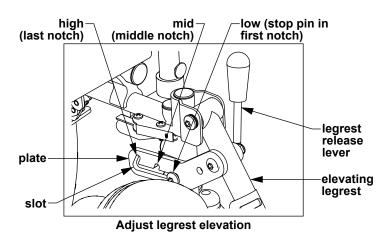
Moving the release lever forward raises the plate notch from the stop pin, allowing the plate slot to move over the stop pin and change position. Moving the release lever rearward lowers a plate notch onto the stop pin and locks it in place.
